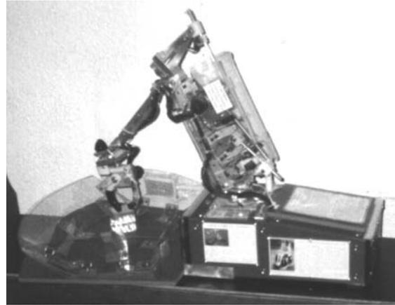
**Figure 8:** Facial feature controlled robot arm activity center moves simple objects in response to eyebrow and nostril movement.
