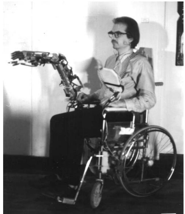
**Figure 3:** Our first feature controlled robotic wheelchair.
