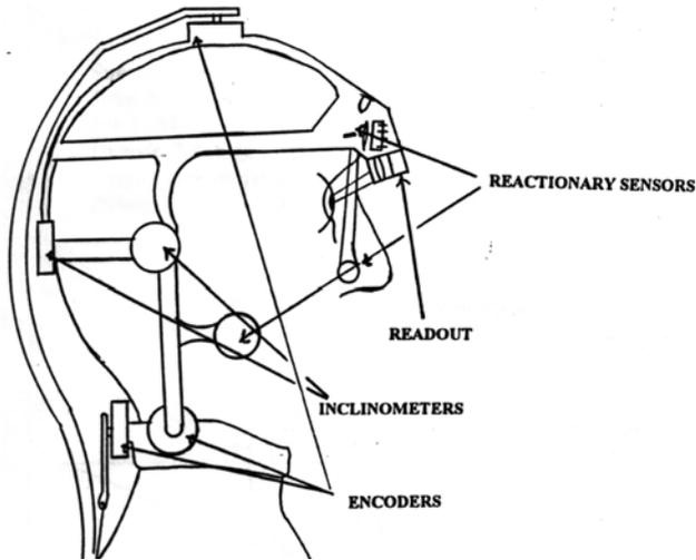
**Figure 6:** Feature & gesture control design. Feedback provided by a readout and lens above the left eye.
